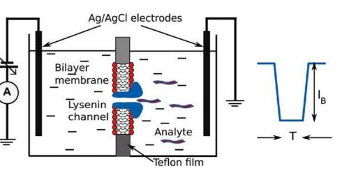
(the fluid within the cell). Once lysenin is inserted into the membrane, it forms stable nano-sized channels, or pores, through the hydrophobic, or waterrepelling, cell wall. Prof Fologea and his colleagues use these channels to their advantage, by recreating the way the protein forms the pores in the cell wall.
