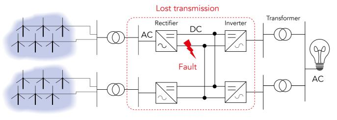
Without a circuit breaker (above), a fault prevents the flow of current acrosss the whole circuit. With a DC circuit breaker (below), a fault can be isolated, allowing current to flow from the remaining wind farms.
