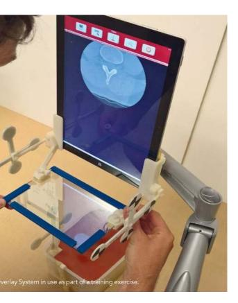
Further, they have developed a calibration method. Two-step calibration takes place away from the patient, and is only required once. The first step is the system calibration, which requires three optical markers. The system is moved through space, and the changes, or transforms, that are registered are recorded using these trackers. These transforms can then be compared and the system can be
