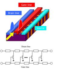
is essentially a pulse oscillator using TWFETs, which could someday render a valuable scheme for reducing phase noise.
