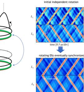
each collision, and so the amplitude of the colliding pulses decrease over time. While an anticlockwise pulse has a slightly smaller amplitude than the clockwise pulse before a collision, the amplitude discrepancy increases after the collision; specifically, the amplitude of the anticlockwise pulse decreases whereas that of the clockwise pulse either increases or remains the same. After several subsequent head-on collisions, the anticlockwise pulse disappears,
