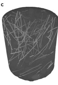
Image A shows a photo of the concrete cylinder sample, which was investigated. Image B shows a slice of 3D CT data in the middle of the sample. Image C reveals the 3D distribution of steel fibres within the self-compacting concrete.
