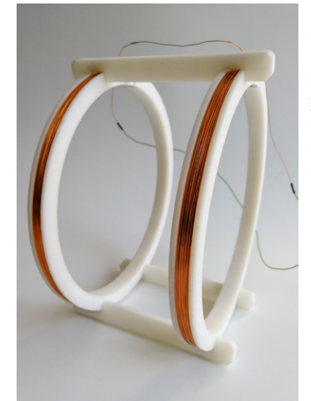
A Helmholtz coil which Dr Scherlag suggests could help patients who are near death.
