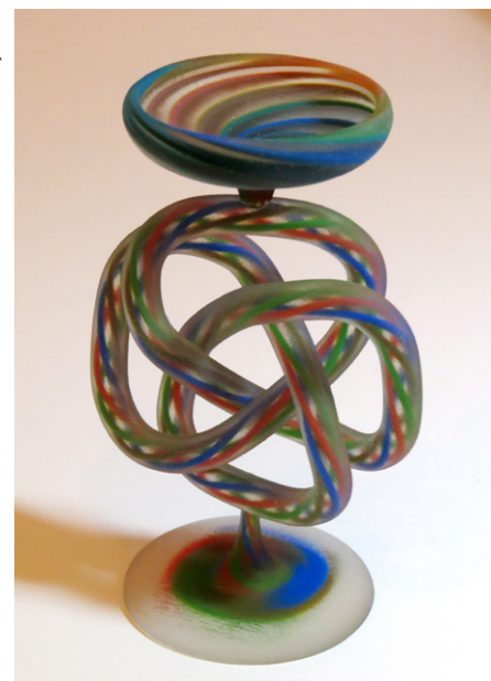
A 3D printed V-rep model made with heterogeneous materials.
