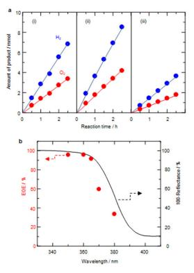
a: Time courses of H<sub>2</sub> and O<sub>2</sub> evolutions on three different photocatalysts: b: AQY(EQY) at several wavelengths
