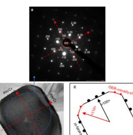
Detailed structure of a SrTiO $_3$ :Al photocatalyst particle with HER and OER co-catalysts.
