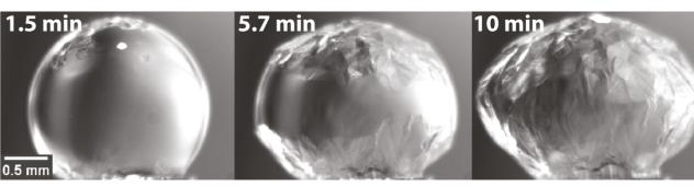
For surfactant concentration below or very close to CMC, hydrate growth showed a planar morphology, moving from both the top and bottom of the water droplet towards the equator, eventually overtaking the shape of the droplet.
