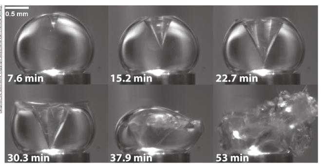
When surfactant was present in concentration higher than CMC, hydrate growth was conical, starting at the top of the water droplet and progressing towards the bottom. When the crystal cone reached the bottom of the droplet, the droplet collapsed.
