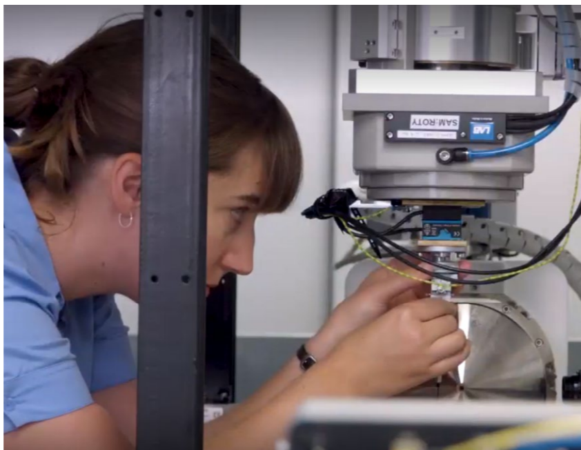
Simone Ferstl is mounting a stained soft-tissue sample on the precision stage in the NanoCT. The mounting of the sample is very crucial to the tomography – a slight move of the sample may make a 3D reconstruction of the acquired data impossible.
