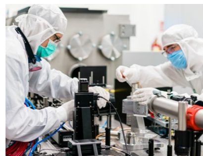
Aligning the LIDT station for testing.
