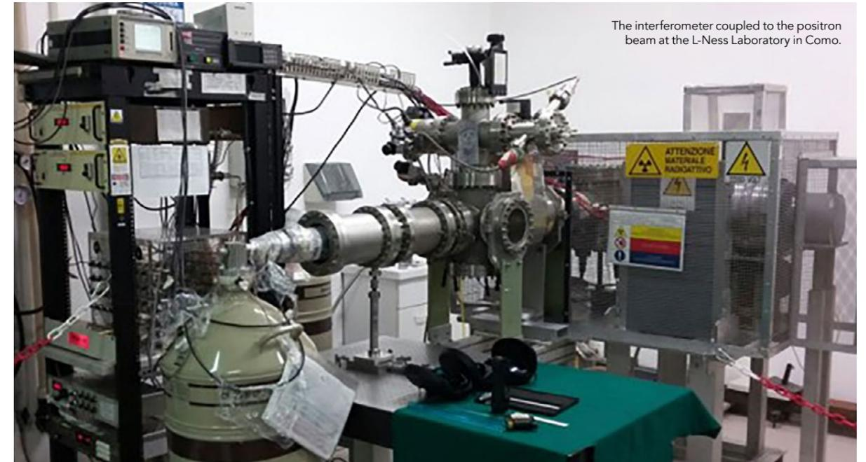
The interferometer coupled to the positron beam at the L-Ness Laboratory in Como.
