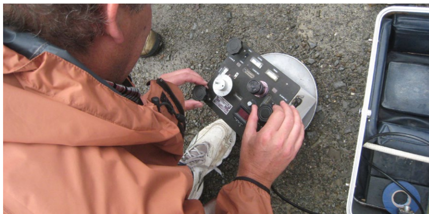
Gravity observations using a portable gravity meter on the shores of Lake Rotomahana.
